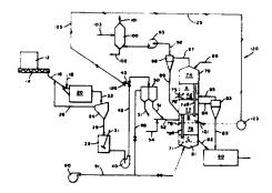
A system for the comminution of coal, slurry formation and feed of the coal slurry to a fluidized bed reactor.
